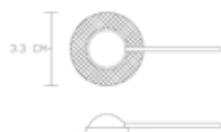
MICRO REMOTE WITH SUTURE DISK 3608-22 (3.3 cm TOTAL DIAMETER)
